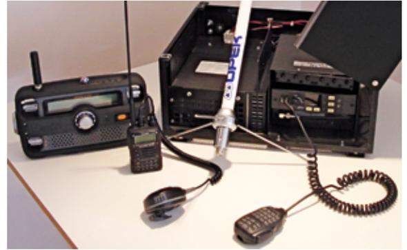
Riviera Association radio network components (from left): emergency radio receivers, handheld radios, and a repeater and antenna, which link the radios together.
